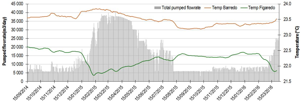
**Figure 9. Corrected and averaged temperature and pumped flowrate for Barredo-Figaredo.**
