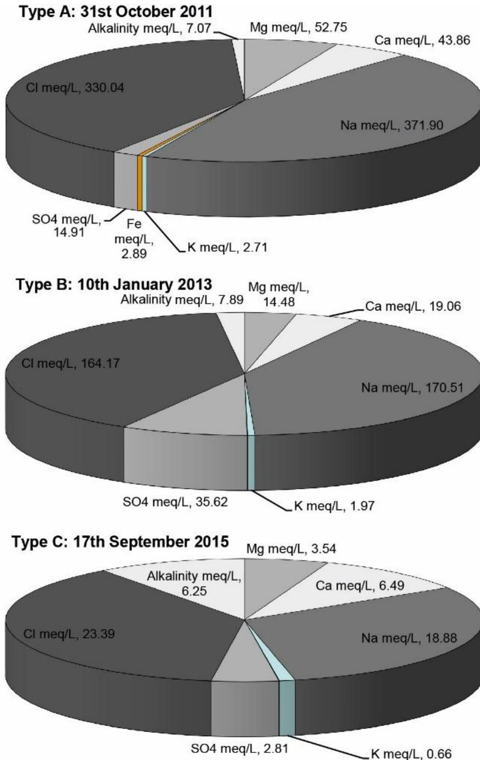
Figure 2. Pie diagrams comparing the major ion (meq/L) composition of the Markham No. 3 Shaft mine water in October 2011 (Type A), January 2013 (Type B) and September 2015 (Type C) (Burnside et al. 2016).
