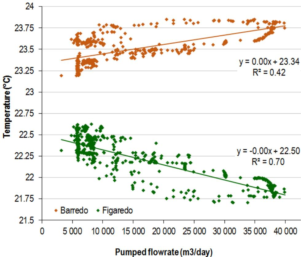
**Figure 10. Direct (Barredo) and Inversed (Figaredo) correlation between pumped rate and temperature at the shaft**
