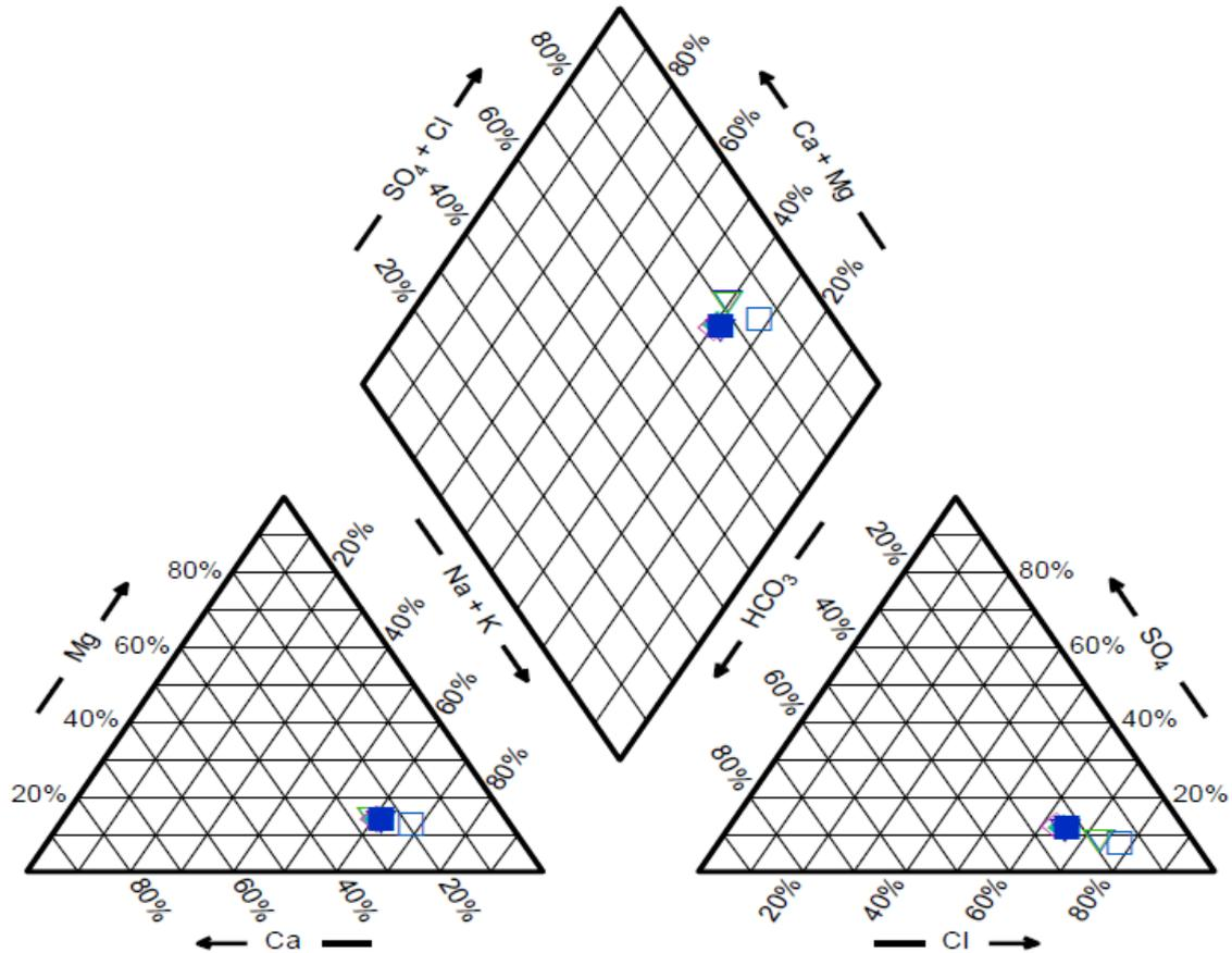
**Figure 4. Piper diagram representation of cation and anion sample distribution for Type C waters.**
