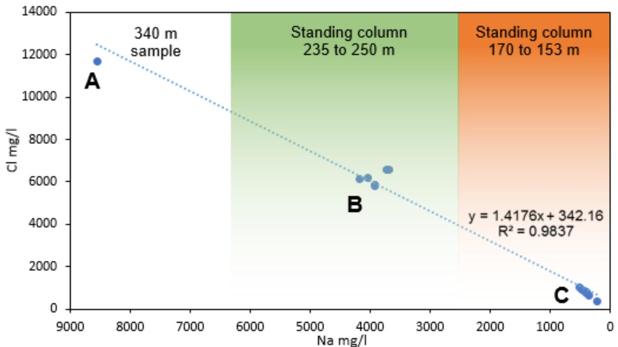
Figure 3. Plot of salinity (Na vs. Cl) evolution throughout alteration of pump depth. Water types labelled as in Fig. 2.
