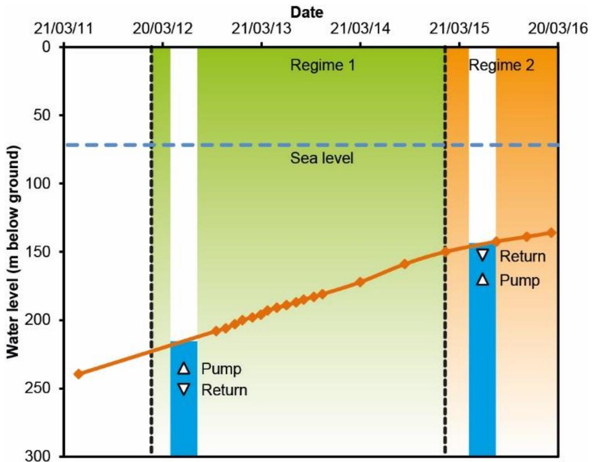
Figure 1. Schematic of the Markham No. 3 Shaft ‘standing column’ heat extraction arrangement, with rise in water level plotted (Burnside et al. 2016).
