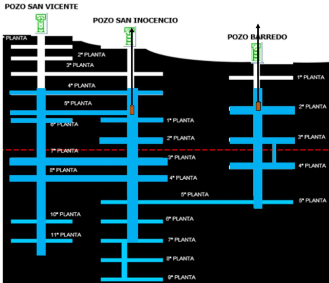
Figure 5. Barredo-Figaredo diagram
