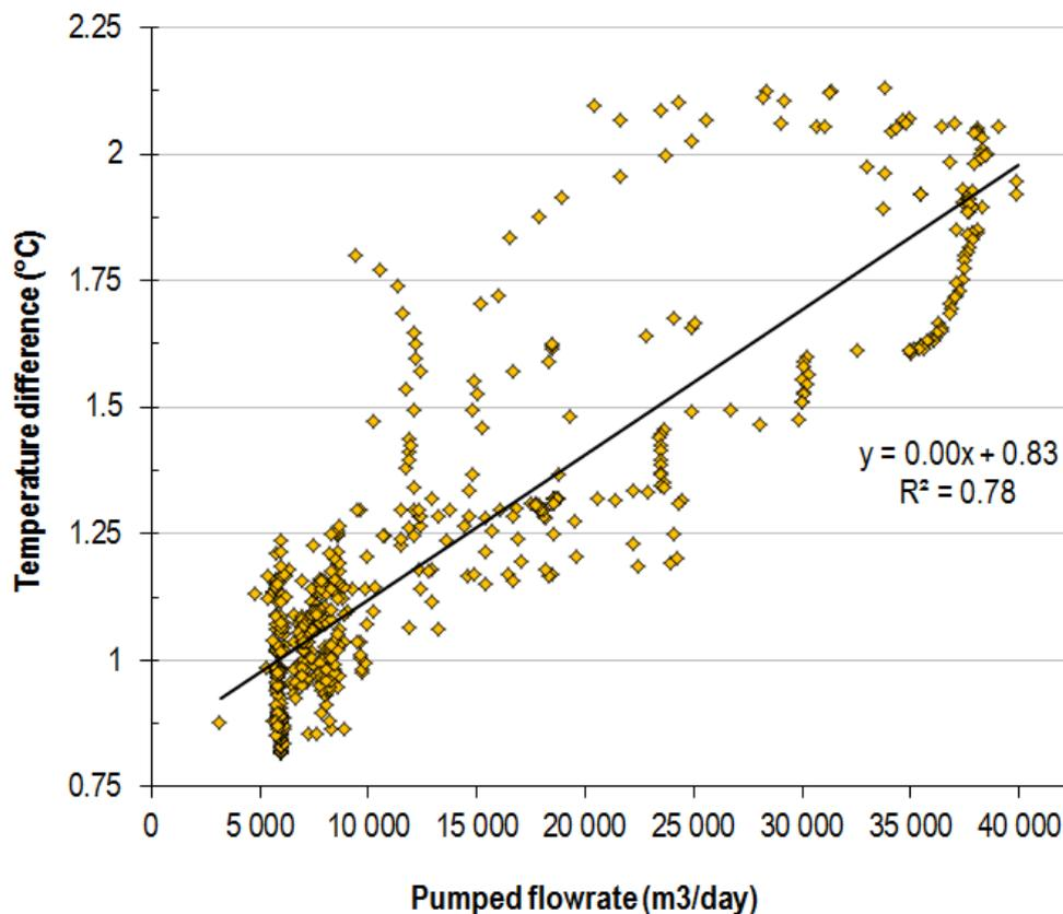
**Figure 11. Temperature difference at Barredo-Figaredo with the pumped flowrate**
