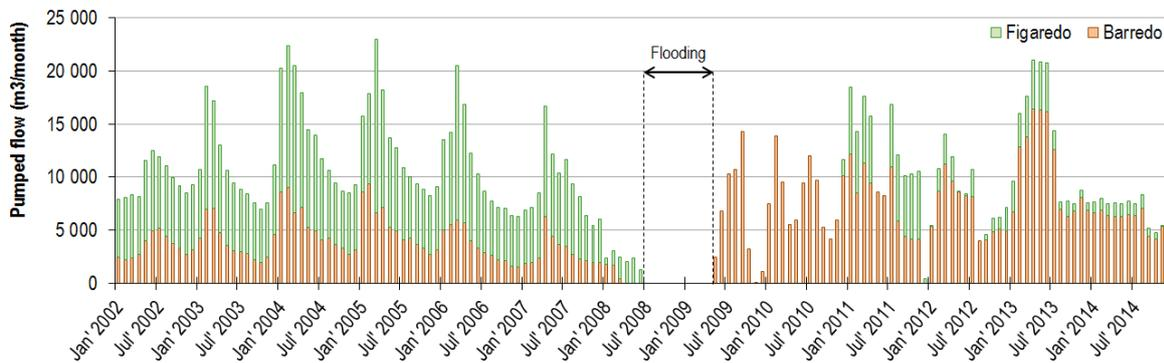
**Figure 8. Temporary register of pumping rates at Barredo-Figaredo from 2002 to 2014**
