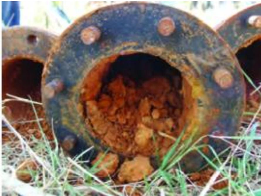
Figure 7. Encrustations in a discharge pipe (Majkic-Dursun et al., 2015)
