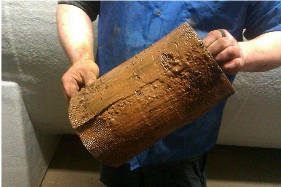
**Figure 16. Filter before cleaning.**
