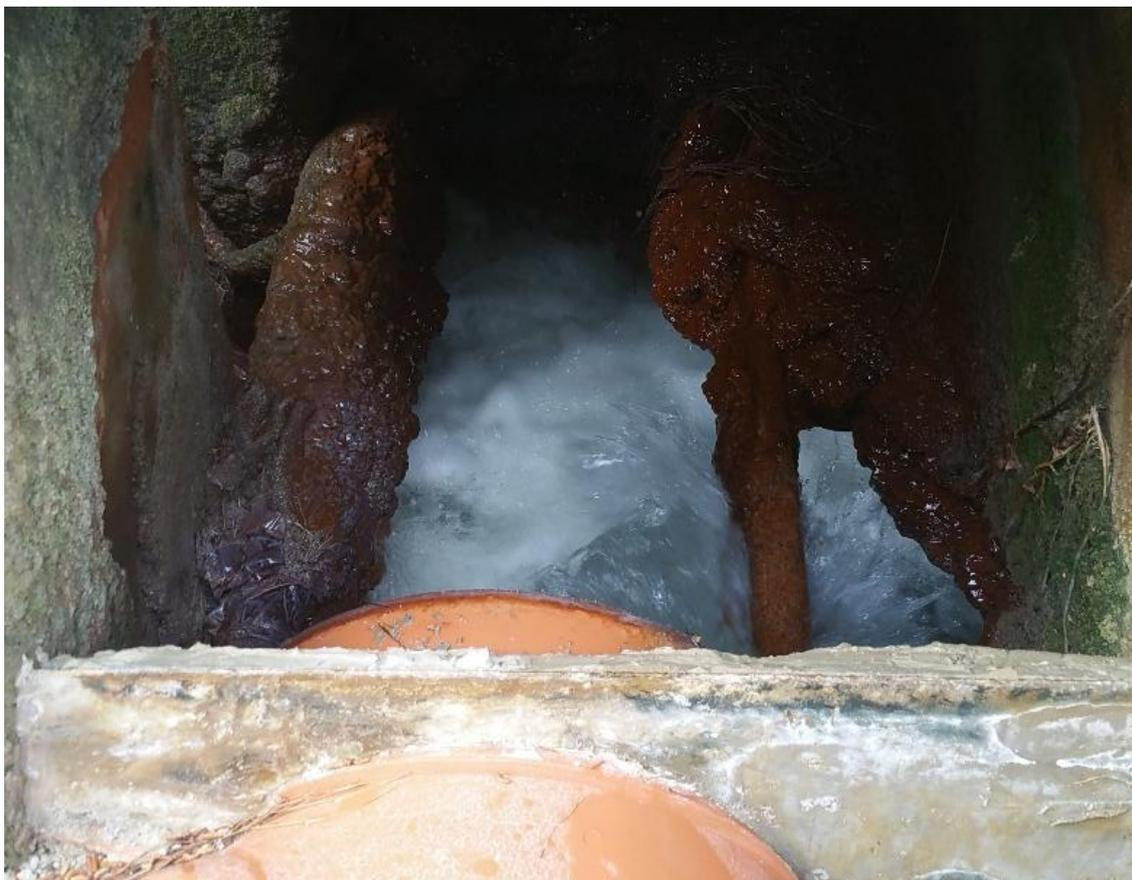
**Figure 2. Ochre deposit in mine water discharge in Barredo (Spain)**
