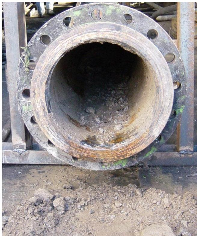
**Figure 15. Depositions inside a pumping conduction**
