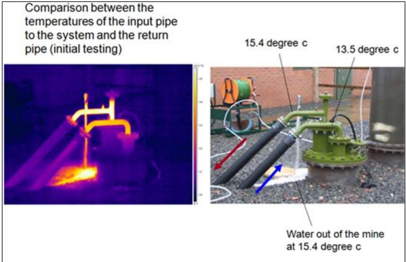
Figure 6: Thermographic image of mine water flow and return.
