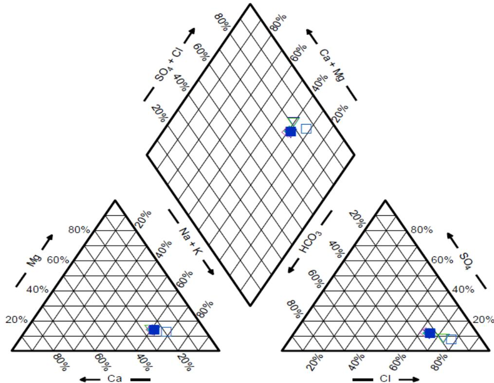
Figure 13: Piper diagram representation of cation and anion sample distribution for Type C waters
