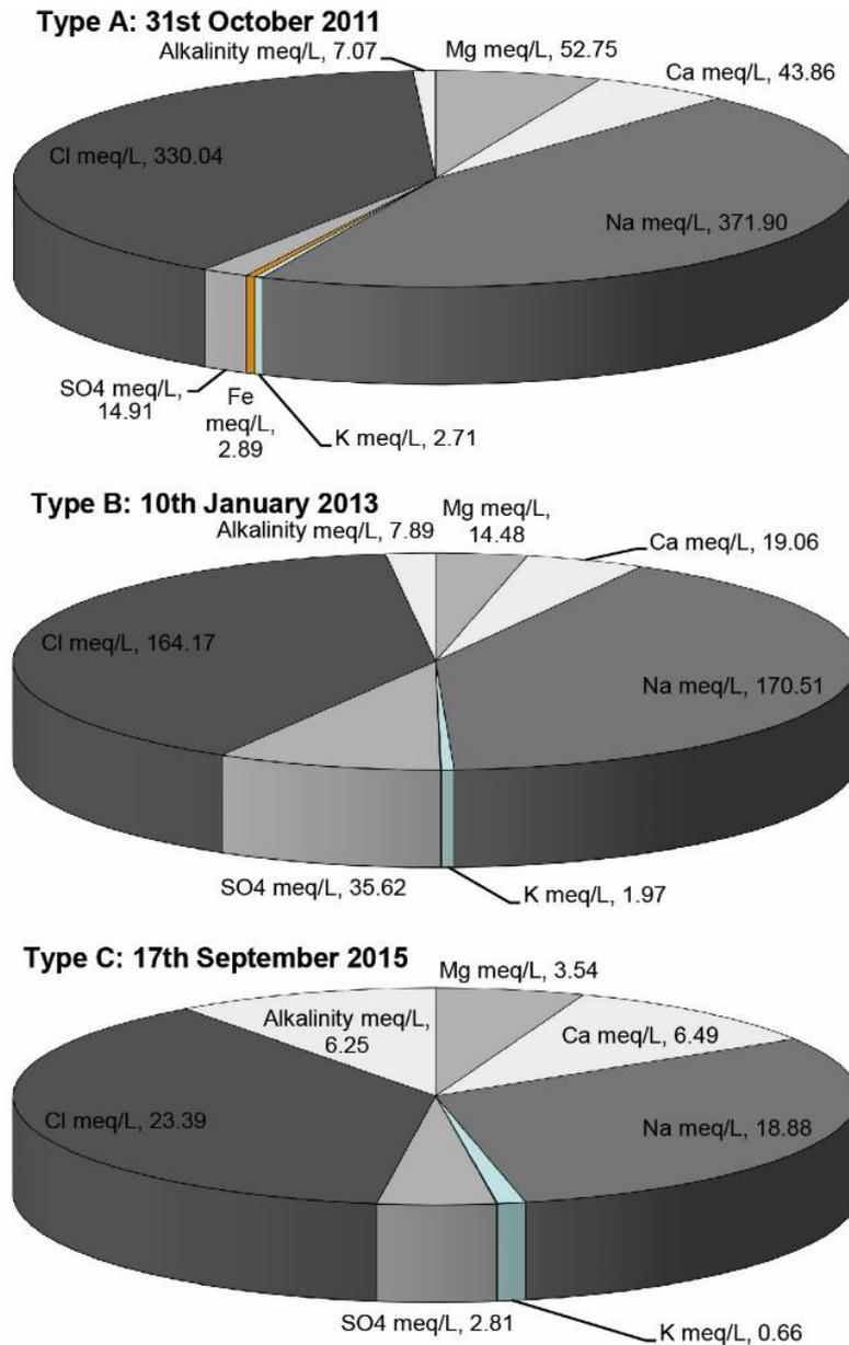
**Figure 11: Pie diagrams comparing the major ion (meq/L) composition of the Markham No. 3 Shaft mine water in October 2011 (Type A), January 2013 (Type B) and September 2015 (Type C) (Burnside et al. 2016).**
