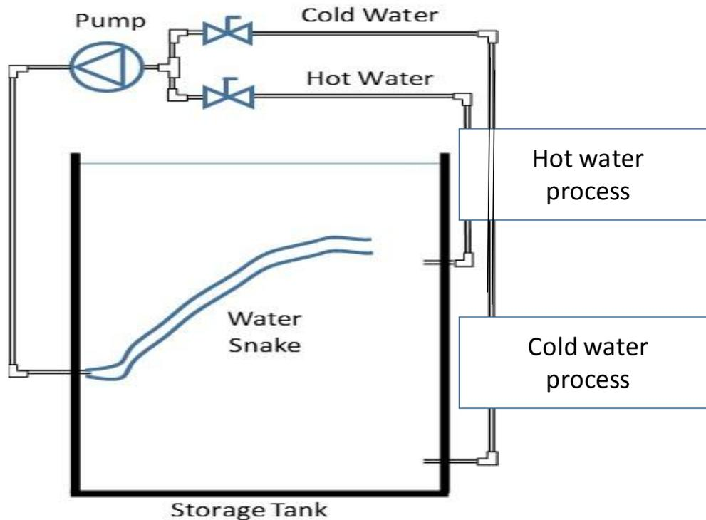
Figure 22: A schematic diagram of the automated experimental test rig.
