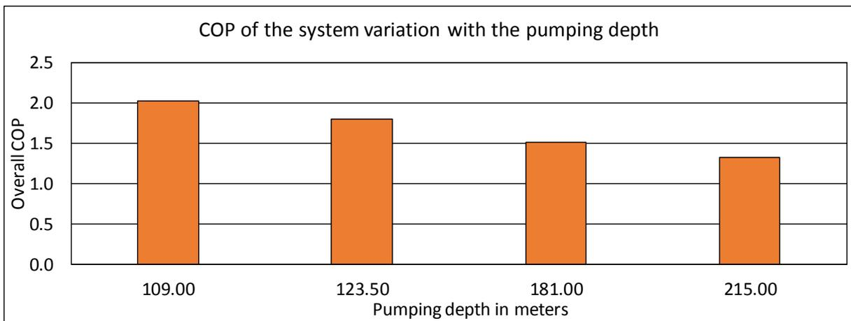
Figure 14: Improvement in the overall COP due to the rising mine water levels
