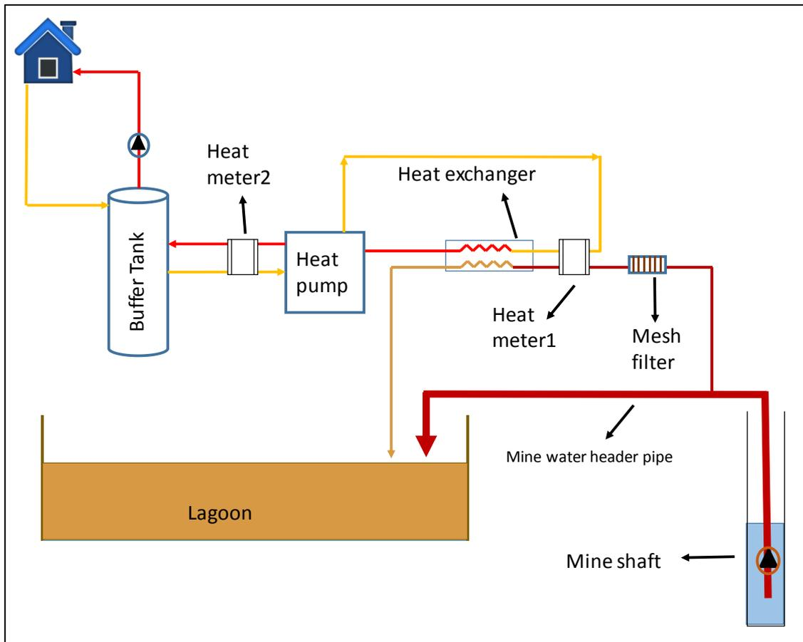
Figure 4: Schematic of the Markham system
