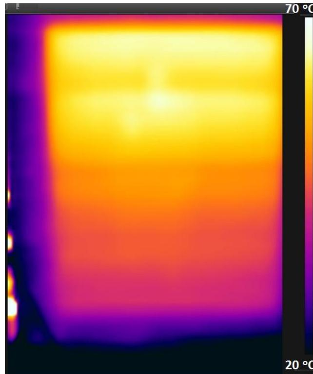
Figure 23: : Infrared thermal image of the fully stratified tank taken after using the water snake.
