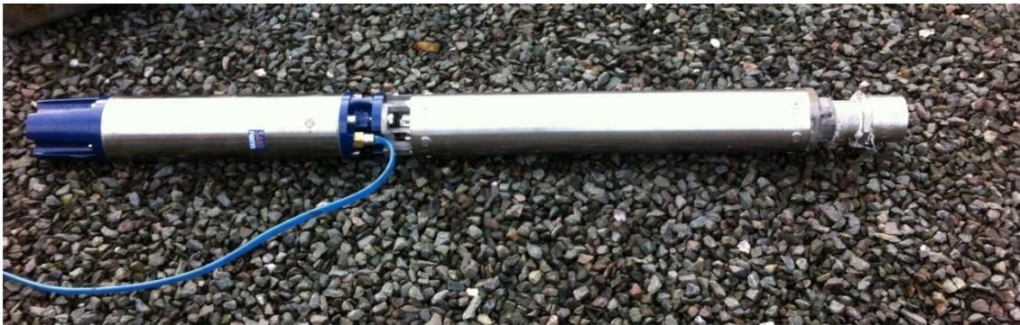
**Figure 9: Borehole pump**
