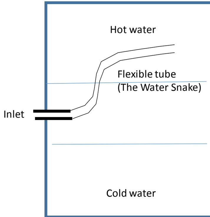
**Figure 21: A schematic diagram that shows the movement of the water snake to the proper water layer that match the inlet water temperature.**
