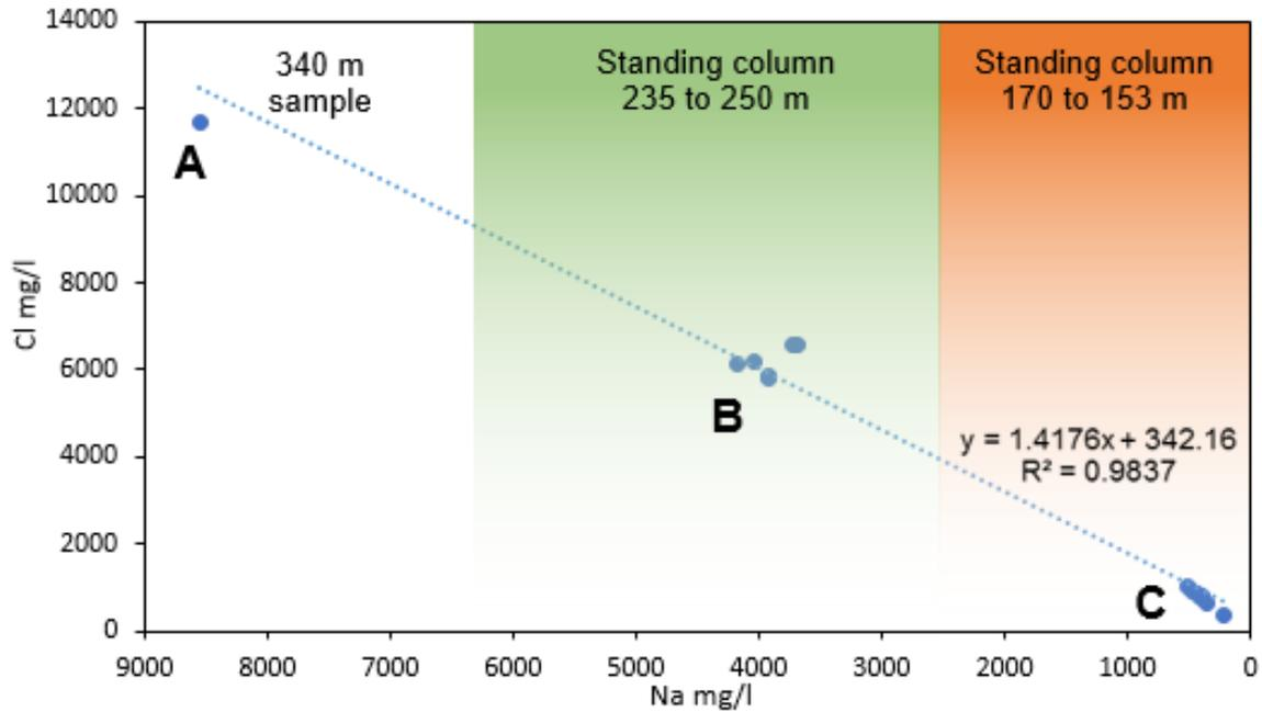
Figure 12: Plot of salinity (Na vs. Cl) evolution throughout alteration of pump depth. Water types labelled as in Figure 11
