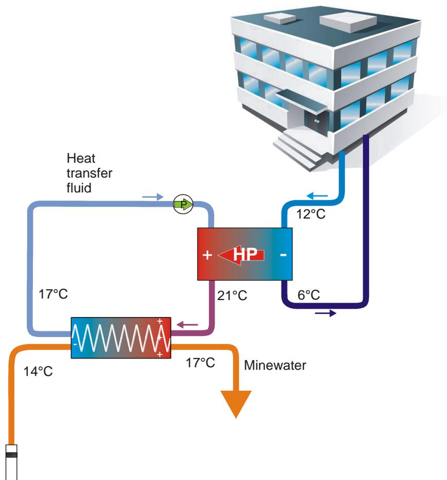
**Figure 3.1.** Highly schematic diagram of simple cooling of a conventional 6°/12°C air conditioning circuit using a heat pump and mine water as a sink.
