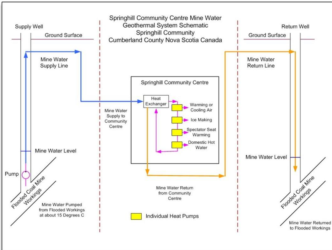
**Figure 7.3. Springhill Community Centre mine water geothermal system schematic** (provided by Brian Herteis)
