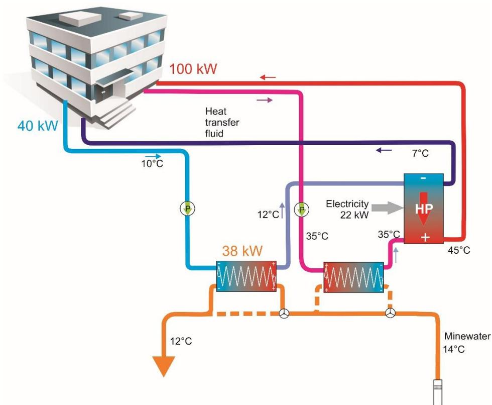
**Figure 3.5 (top).** A schematic example of a mine water heat pump performing heating, with a subsidiary cooling load from the evaporator. Here the  $COP_H = 100/22 = c. 4.5$ , while the effective COP ([heating effect + cooling effect] / electricity) is  $140/22 = 6.3$ . **(bottom)** Topologically, the same circuit, but employing two heat exchangers to facilitate switching between heating-dominant and cooling-dominant modes. Dashed orange = inactive minewater circuit.
