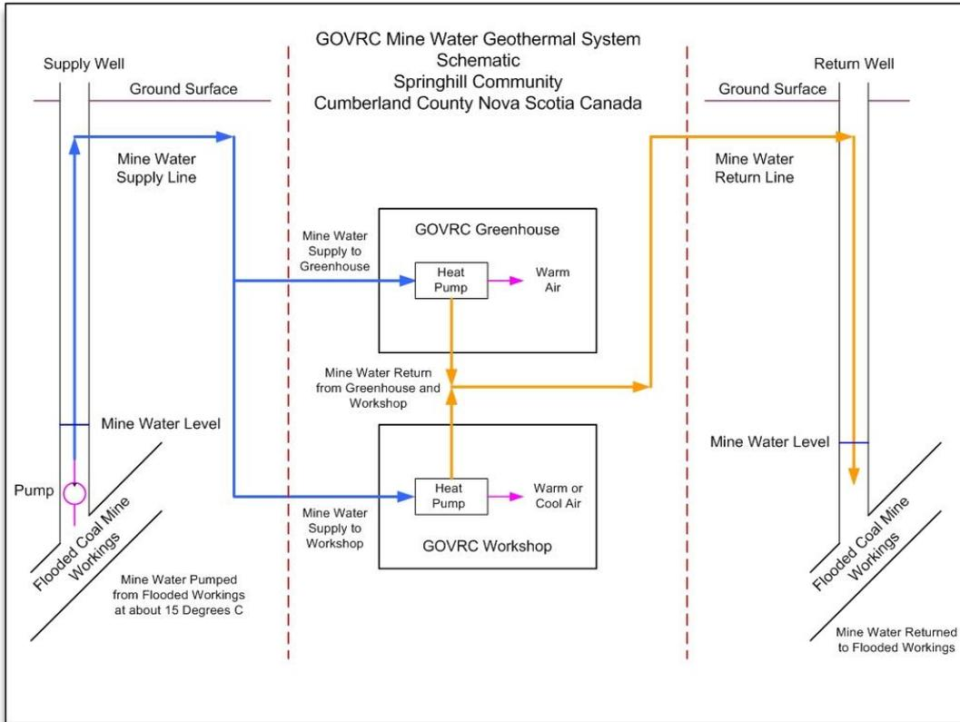
**Figure 7.2. GOVRC mine water geothermal system schematic** (provided by Brian Herteis)
