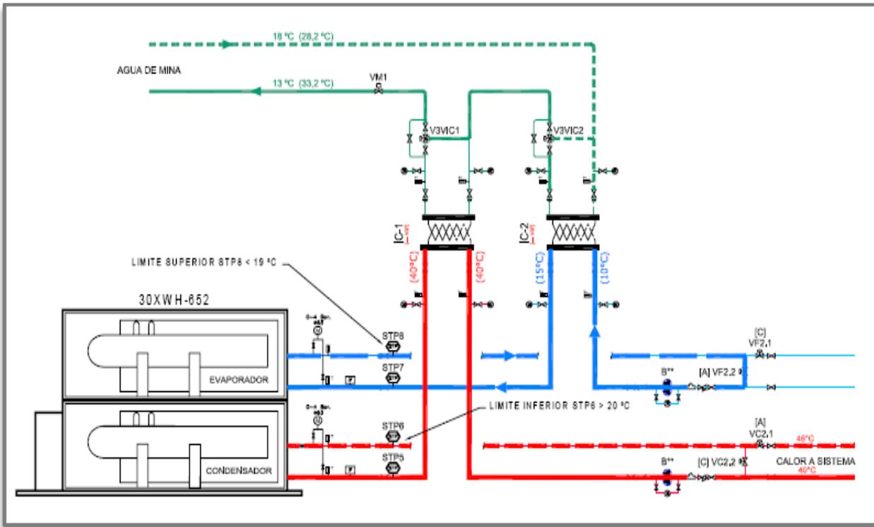
**Figure 6.12. Heat pump GF2 in heating mode.** The evaporator of the heat pump is coupled to the secondary heat transfer circuit (and thence to the mine water) via a heat exchanger (IC-2).
