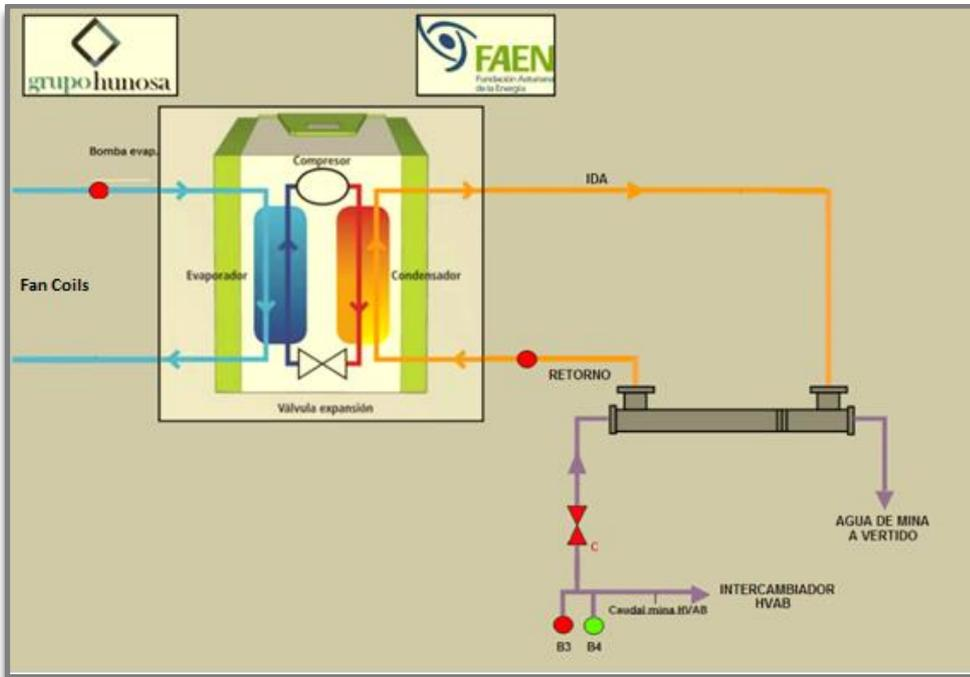
**Figure 6.19. FAEN thermal system in cooling mode.**
