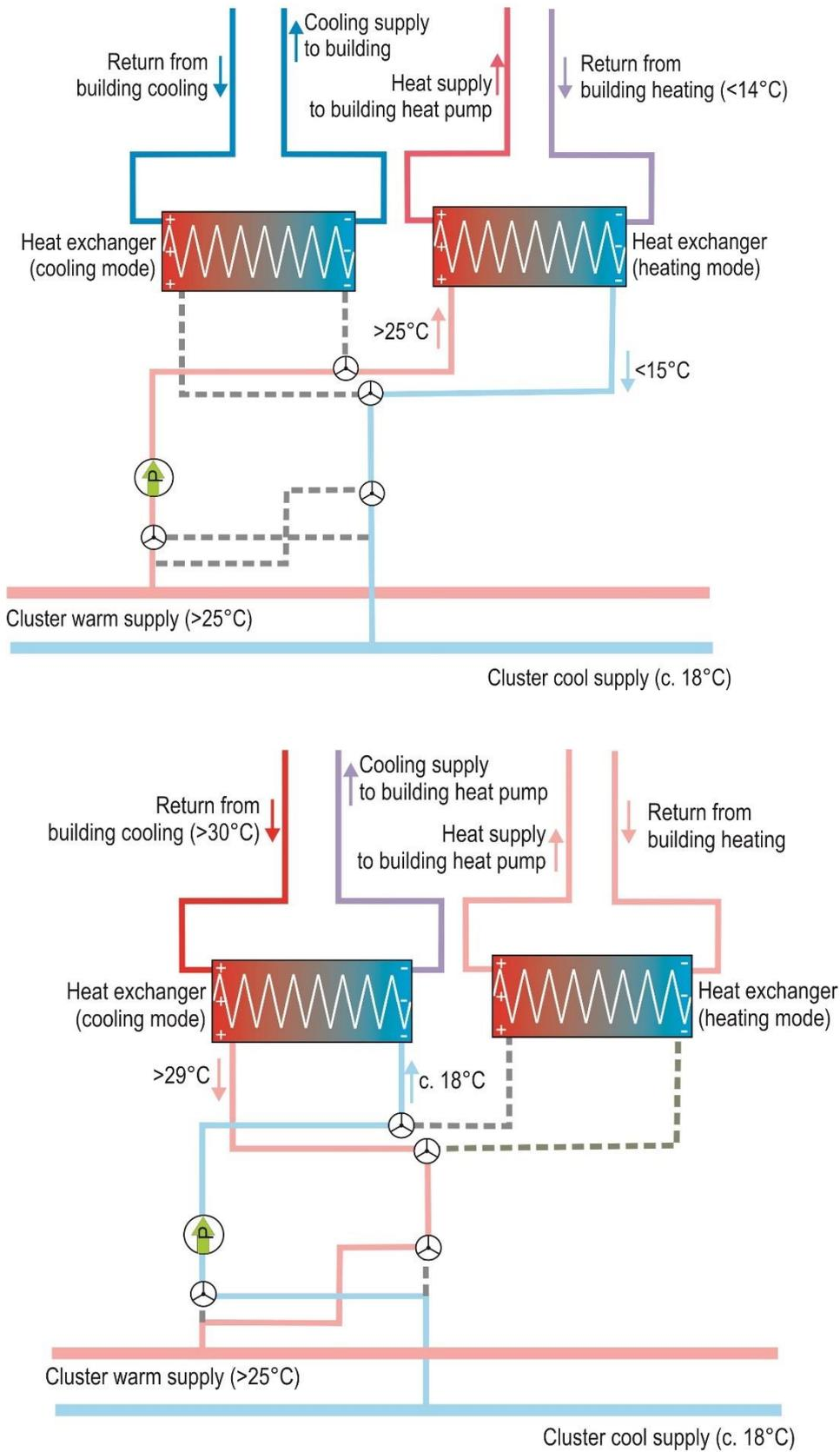
**Figure 8.3. Schematic of heat transfer at Heerlen from secondary (cluster) to tertiary (consumer building heat pump) levels, in (top) heating and (bottom) cooling modes, using double heat exchangers. Grey dashed lines indicate temporarily not in use.**
