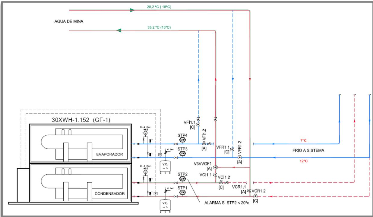
**Figure 6.8. Heat pumps GF1 and GF3 in cooling mode.** V.FI1.1 = closed; VFR1.1 = closed; VCR1.2 = closed; VCI 1.2 = closed. *Frio a Sistema* = building cooling circuit, *Agua de Mina* = secondary heat transfer circuit coupled to mine water.
