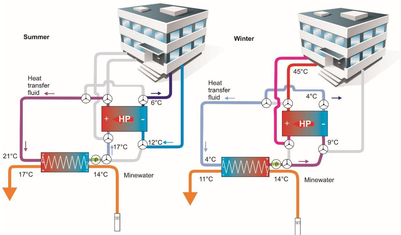
**Figure 3.3.** Schematic diagram of reversible heating and cooling achieved by altering flow in the building and intermediate heat transfer circuits. In this case, the fluid in all of the circuits should be compatible and similar.
