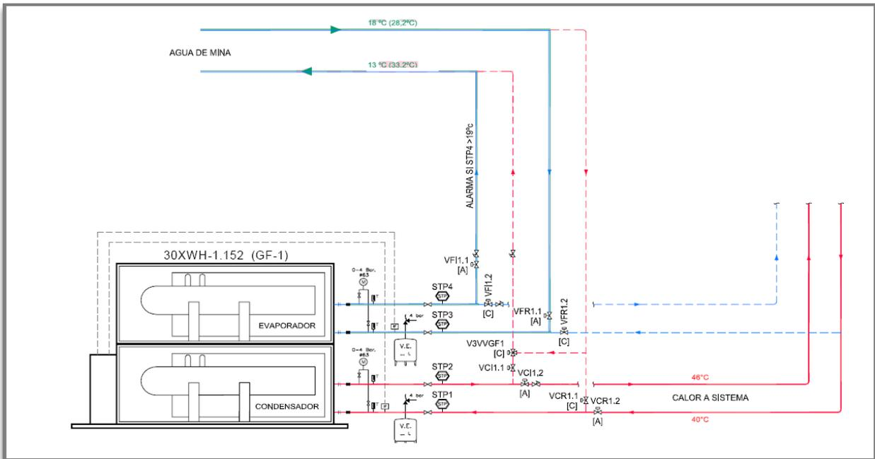
**Figure 6.9. Heat pumps GF1 and GF3 in heating mode.** V.FI1.2 = closed; VFR1.2 = closed; VCR1.1 = closed; VCI 1.1 = closed. *Calor a Sistema* = building heating circuit, *Agua de Mina* = secondary heat transfer circuit coupled to mine water.
