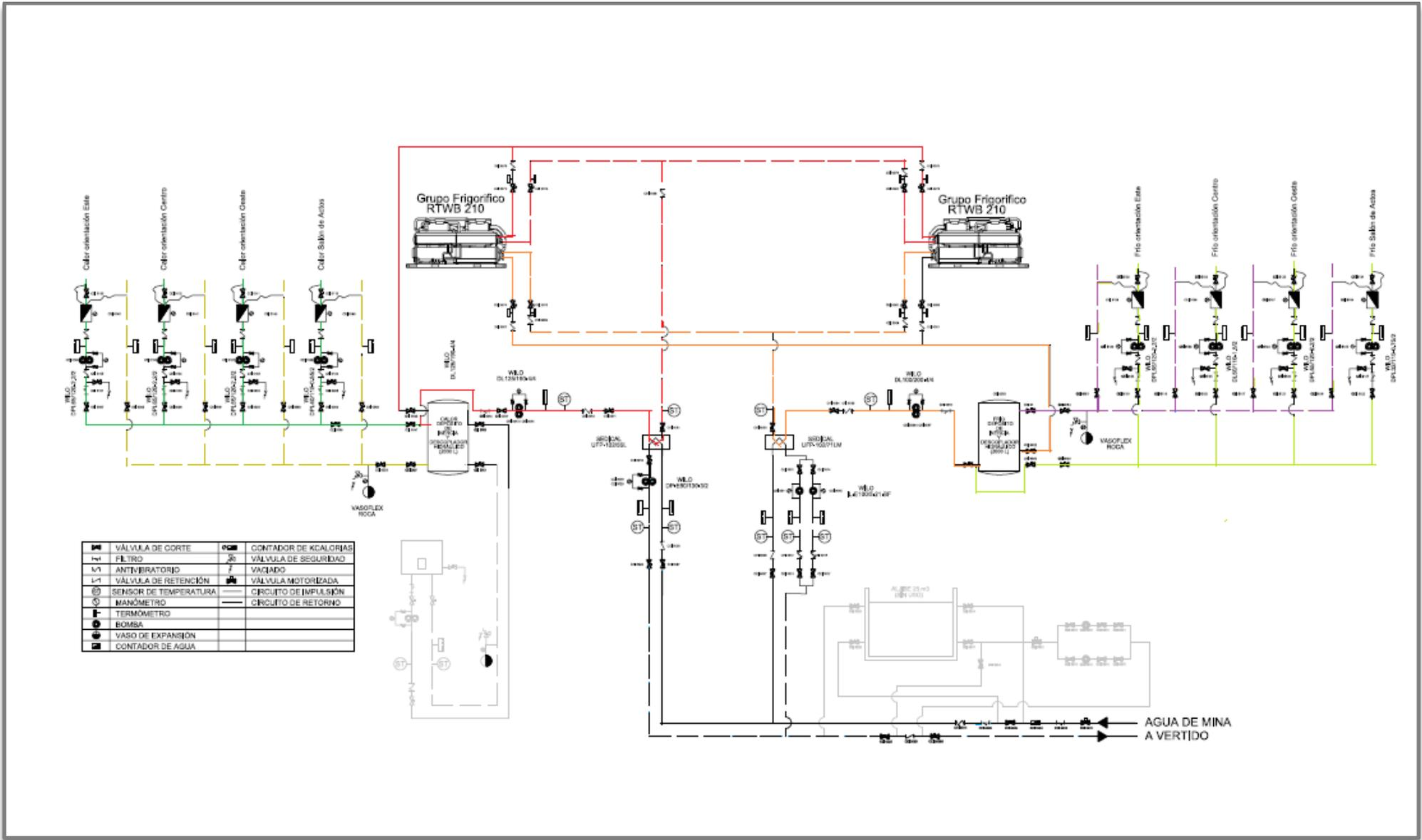
**Figure 6.4. The University heat pump system in heating/cooling mode.** Blue line: mine water, orange = evaporator circuit, red = condenser circuit, lime green = cooling flow, purple = cooling return, green = heating flow, yellow = heating return.
