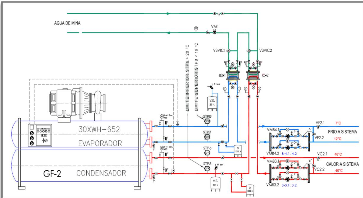
**Figure 6.10. Heat pump GF2.** This can operate in three modes: cooling only, heating only, both cooling and heating. The heating circuit operates at a flow/return temperature of c. 46/40°C, the cooling circuit at c. 7/12°C.
