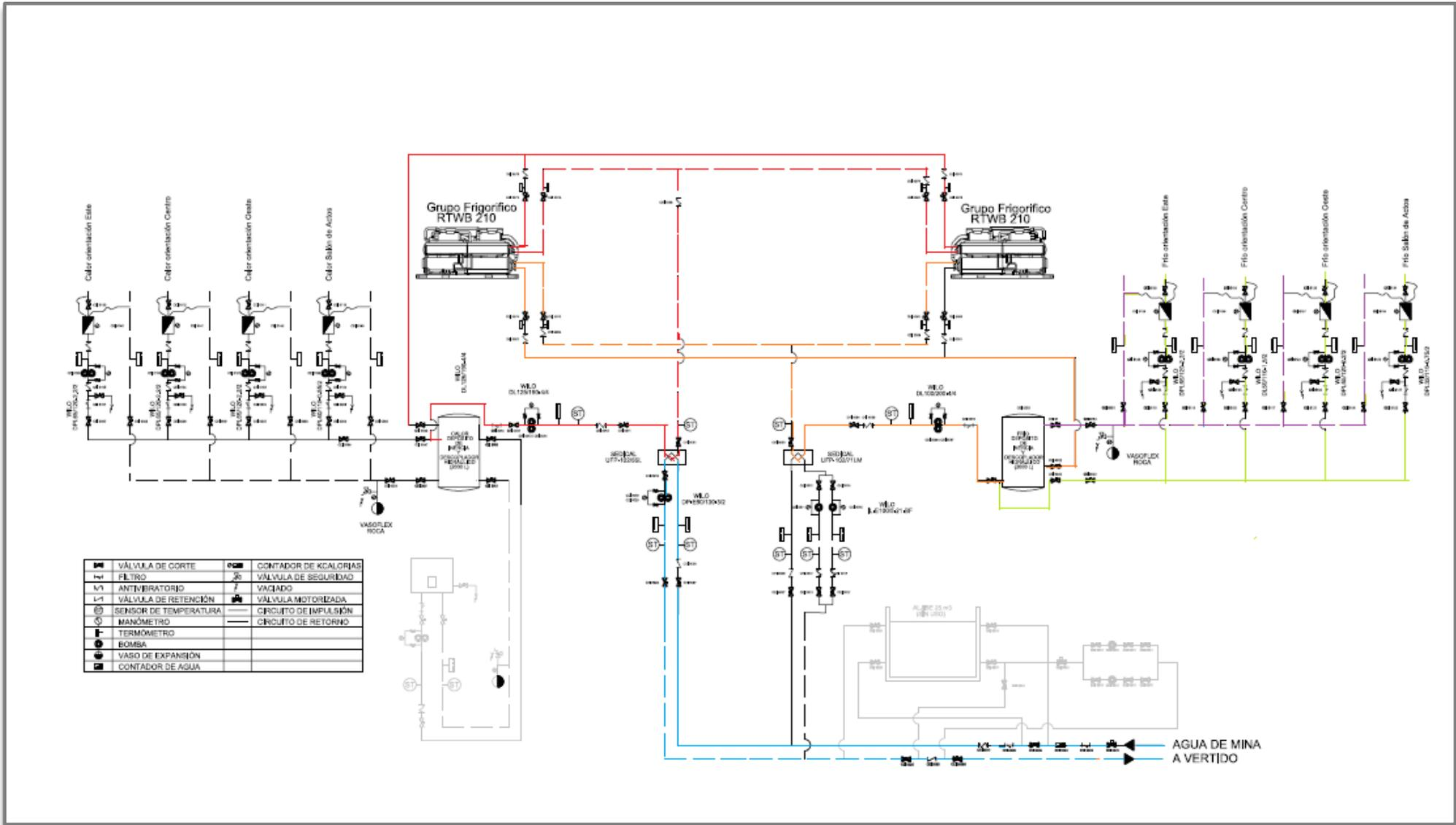
Figure 6.3. The University heat pump system in cooling mode. Blue line: mine water, orange = evaporator circuit, red = condenser circuit, green = cooling flow, purple = cooling return.
