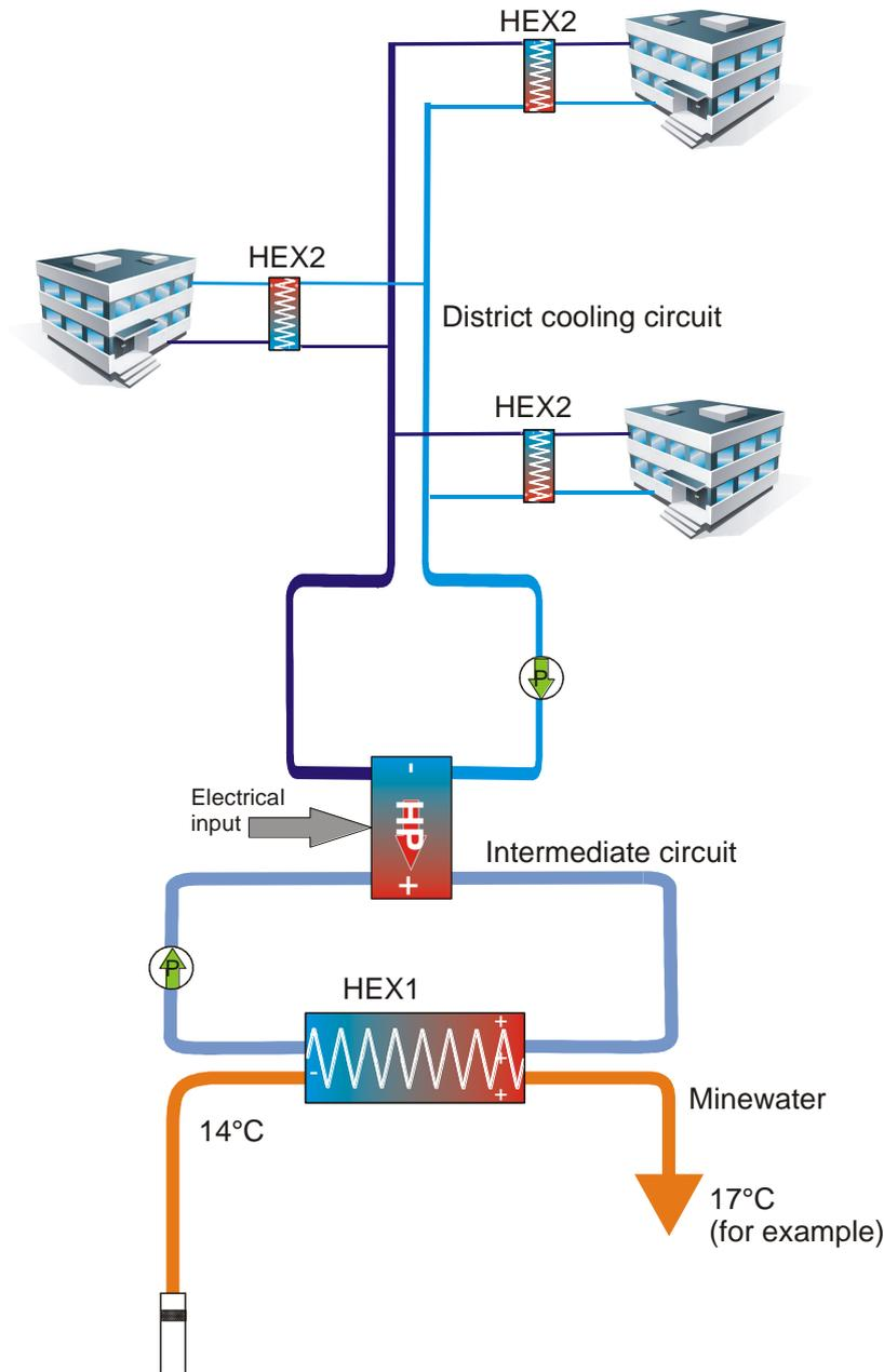
**Figure 4.3. A centralised district cooling system.** Temperatures are indicative examples only. HEX1 is a primary prophylactic heat exchanger. If the mine water is of benign enough quality, it could arguably be circulated directly through the condenser of the heat pump. HEX2 are secondary heat exchangers, which serve to hydraulically separate each consumer from the network.
