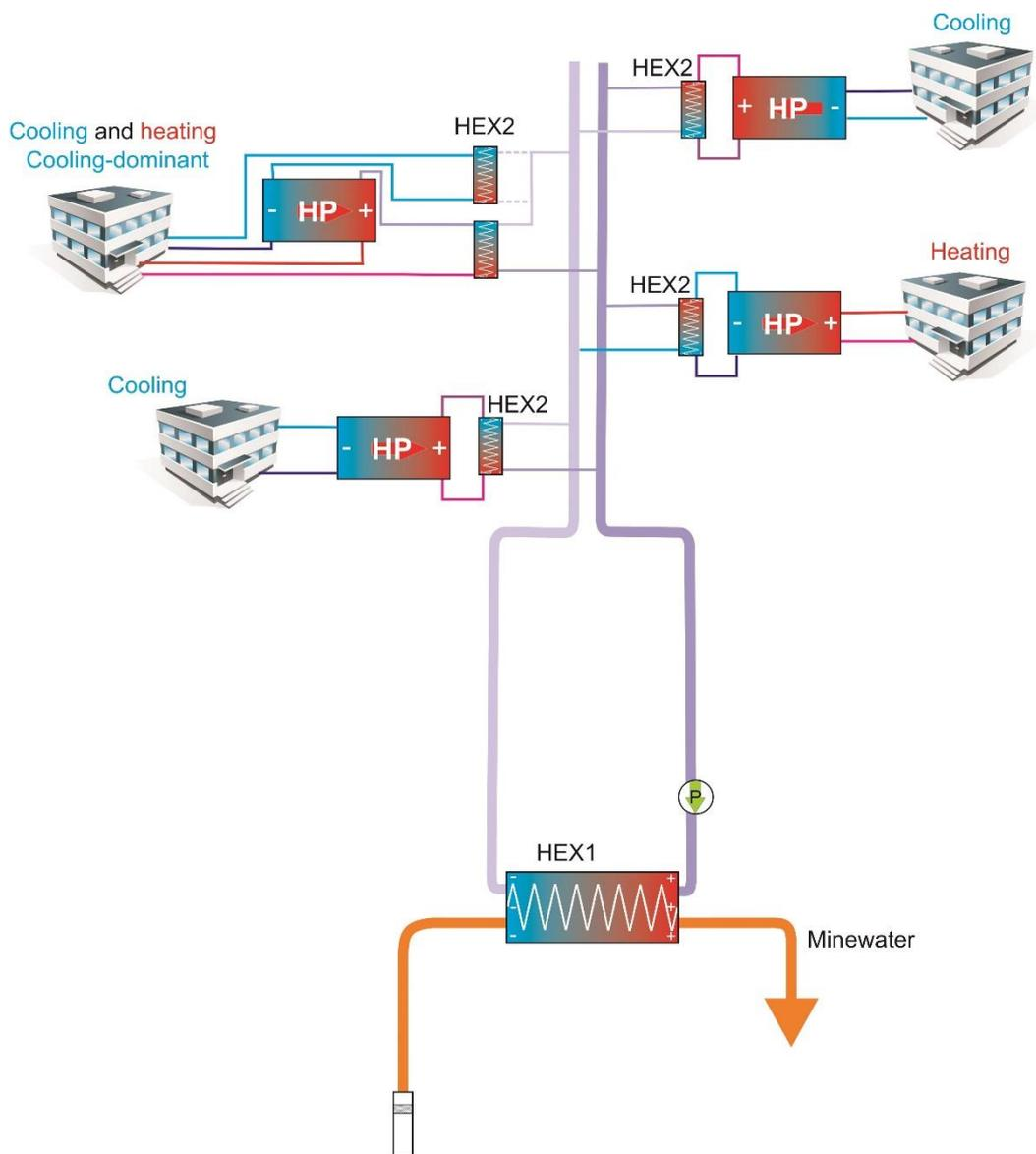
**Figure 4.5. A decentralised district cooling / heating system, where secondary heat exchangers separate the consumers’ heat pumps from the district heating/cooling network.** HEX1 is a primary prophylactic heat exchanger. HEX2 are the secondary heat exchangers. Note that one consumer is using its heat pump to perform space heating, two to perform space cooling. One consumer has a system employing double heat exchangers, enabling simultaneous or reversible cooling and heating.
