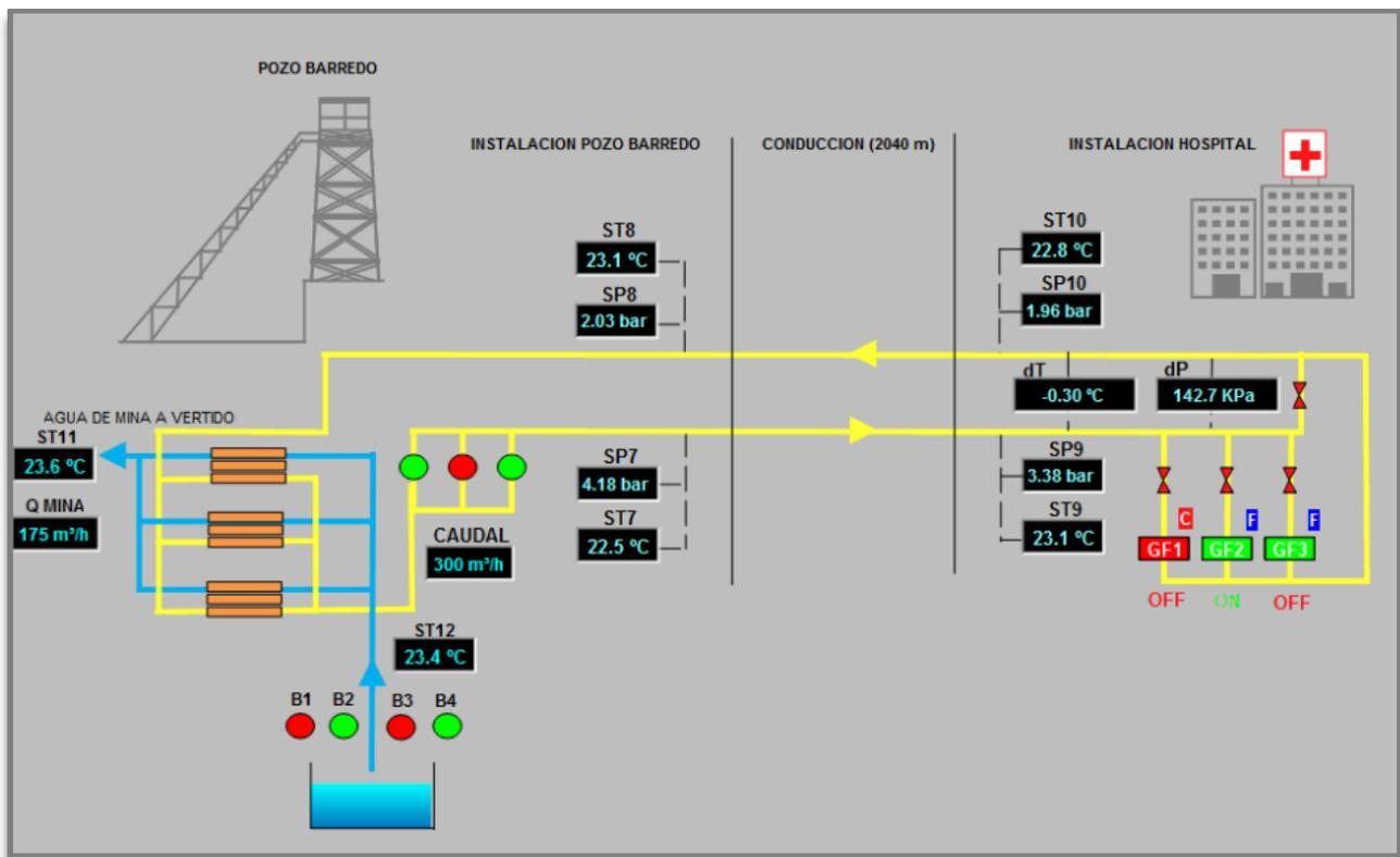
**Figure 6.7. Digital monitoring snapshot of Barredo hospital system** (blue = mine water, yellow = secondary heat transfer circuit to hospital, B1-B4 = submersible pumps in shaft, GF1-GF3 = heat pumps, C = *calor* [heat]; F = *frio* [cooling])
