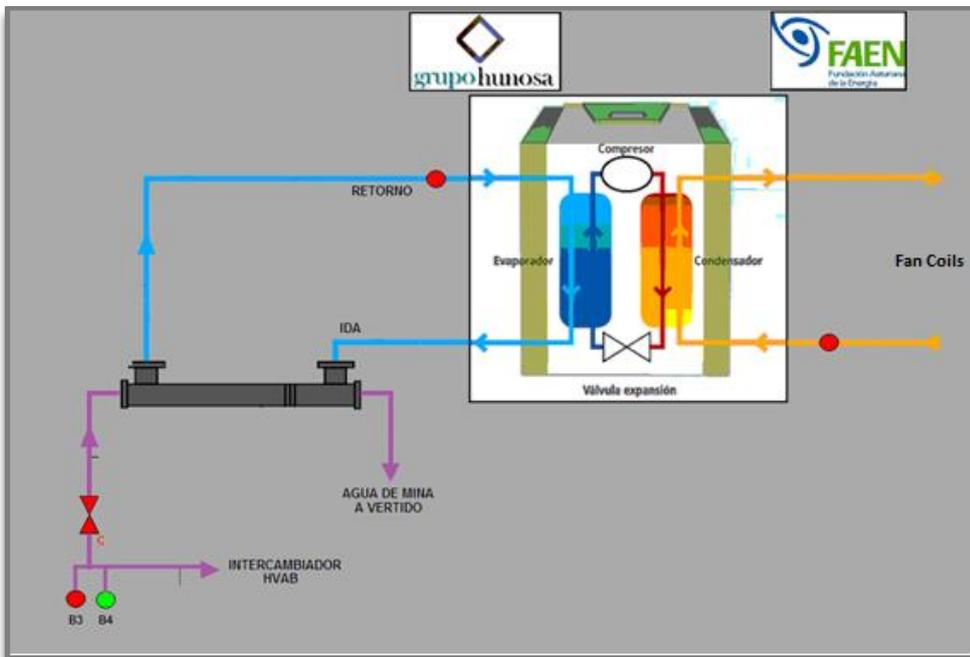
**Figure 6.18. FAEN thermal system in heating mode.** *Intercambiador HVAB* = hospital heat exchanger, *Agua de mina a vertido* = mine water to discharge
