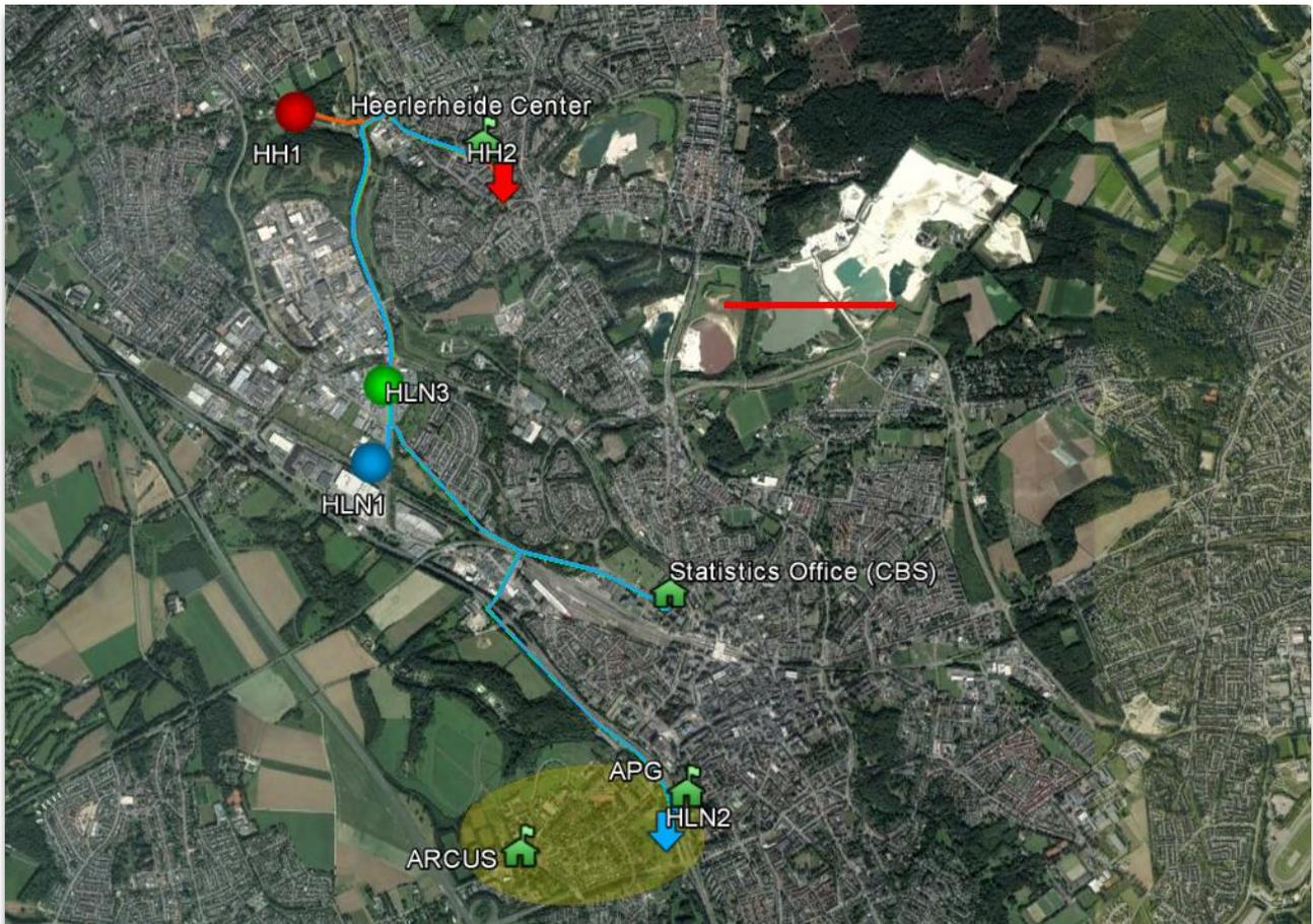
**Figure 8.2. Mijwater 2.0 as of 2013**, showing HH2 as a warm reinjection well, and HLN2 as a cool reinjection well, with the yellow ellipse showing the district cluster around ARCUS and APG.
