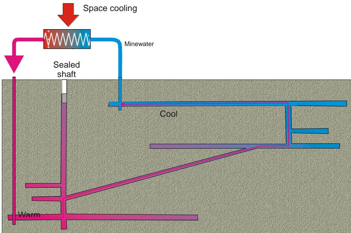
**Figure 4.7. Schematic section of a mine system with shallow workings being pumped to provide space cooling in summer.** The magenta arrow shows the subsurface flow pathway between the reinjection and abstraction boreholes.
