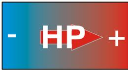
= heat pump (+ or red = warm / condenser side; - or blue = cold / evaporator side)
