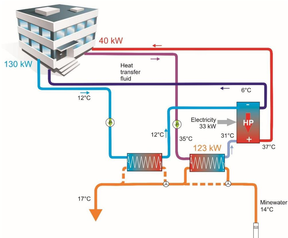
**Figure 3.4 (top).** A schematic example of a mine water heat pump performing cooling, with a subsidiary heating load from the condenser. Here the  $COP_c = 130/33 = c. 3.9$ , while the effective  $COP$  ([heating effect + cooling effect] / electricity) is  $170/33 = 5.1$ . **(bottom)** Topologically, the same circuit, but employing two heat exchangers to facilitate switching between heating-dominant and cooling-dominant modes. Dashed orange = inactive minewater circuit.
