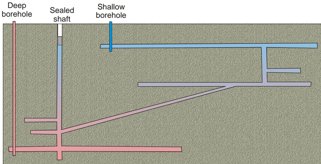
**Figure 5.1. Schematic section of a mine system containing a shallow and deep portion, connected by a drift. The pink shading indicates somewhat warmer mine water, the blue shading, somewhat cooler water.**
