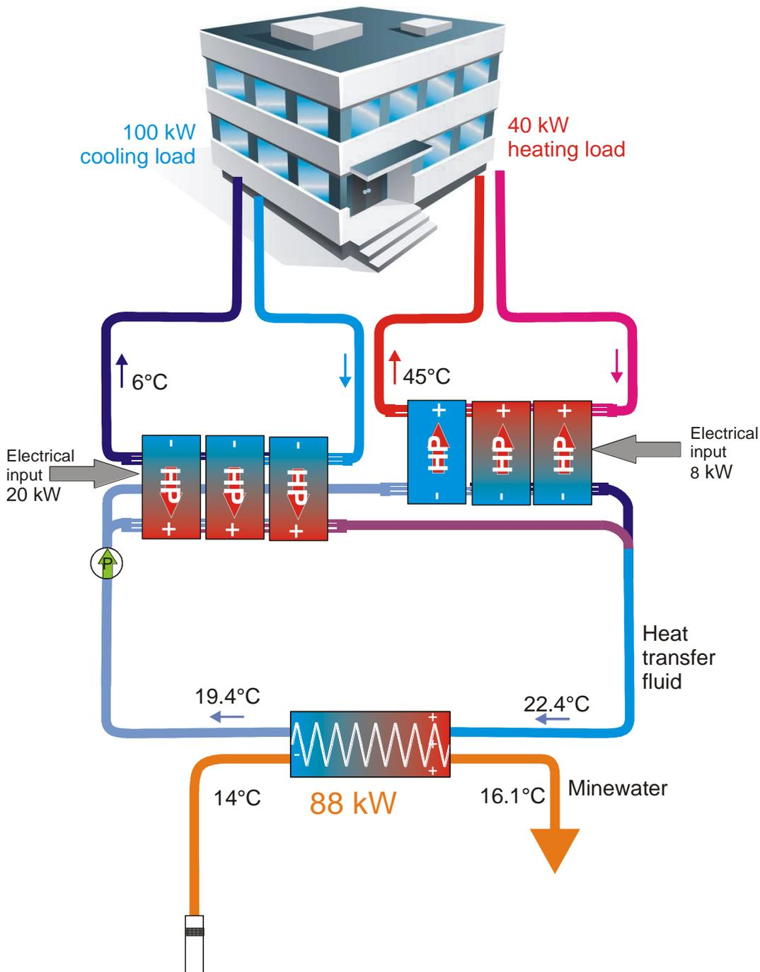
**Figure 3.8.** A schematic example of a mine water heat pump performing cooling and heating, with dedicated parallel arrays of cooling and heating heat pumps. Here, the effective COP ([heating effect + cooling effect] / electricity) is  $140/28 = 5.1$ , slightly lower than the example in Figure 3.7. This arrangement is likely to be more hydraulically efficient, however, and result in energy savings in circulation pumping. The mine water flow in this case is 10 L/s.
