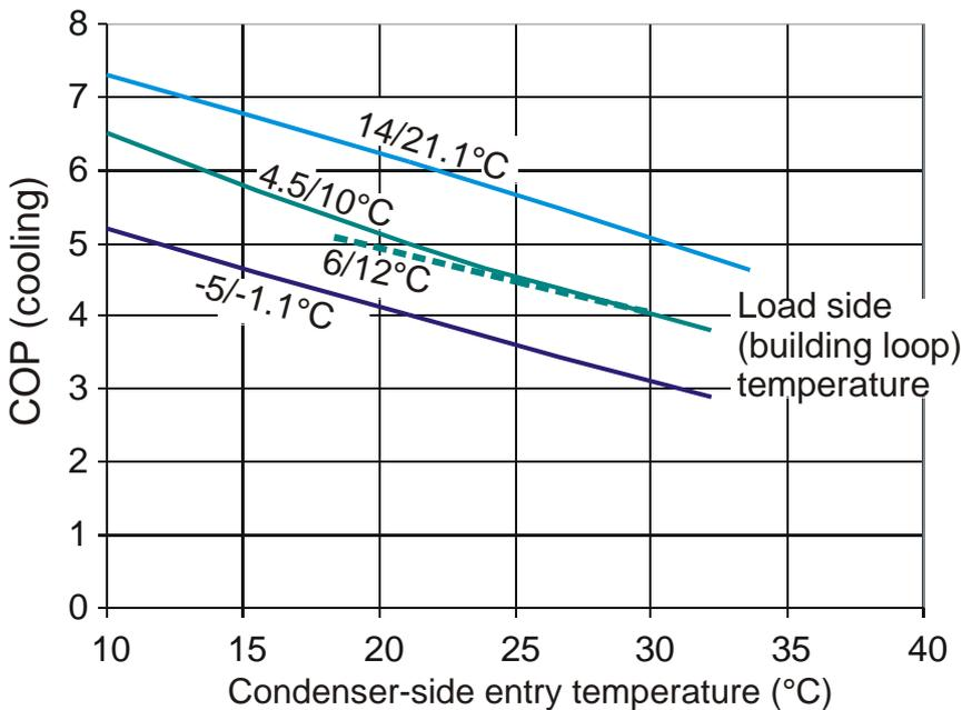
**Figure 3.2.** Dependence of  $COP_c$  on condenser and evaporator temperatures, based on two typical commercial heat pumps (modified after Banks, 2012). These curves will be model-dependent.
