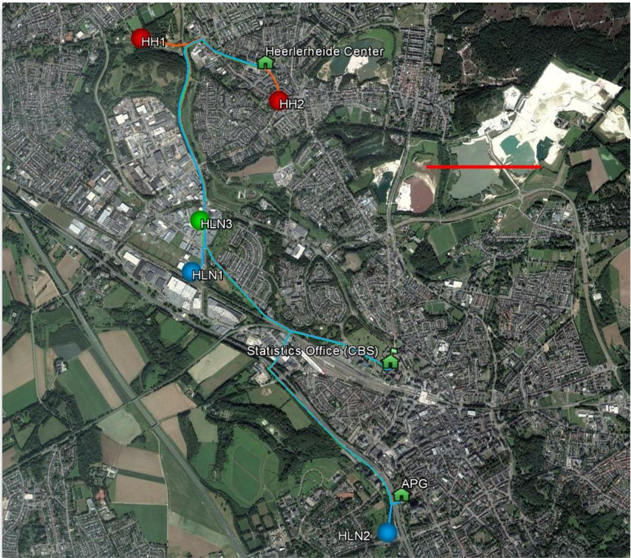
**Figure 8.1. Schematic of Heerlen mine water scheme phase 1.0.** Warm wells and flow pipeline in red, cold wells and flow pipeline in blue, return well and combined return pipe in green. The red bar is a 1 km scale. Based on a schematic from the [www.mijnwater.com](http://www.mijnwater.com) website.
