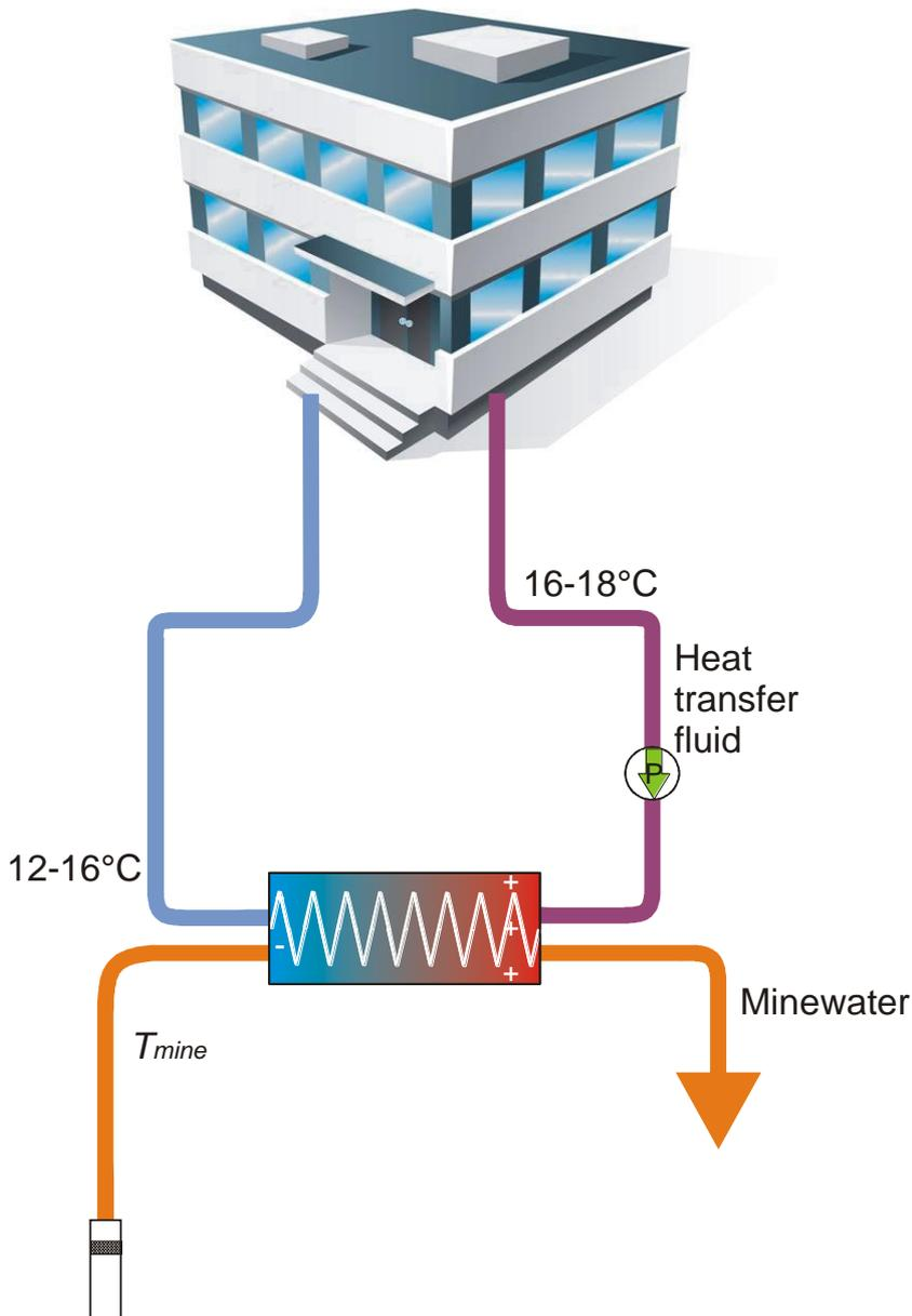
**Figure 2.1.** Schematic of typical passive mine water cooling system
