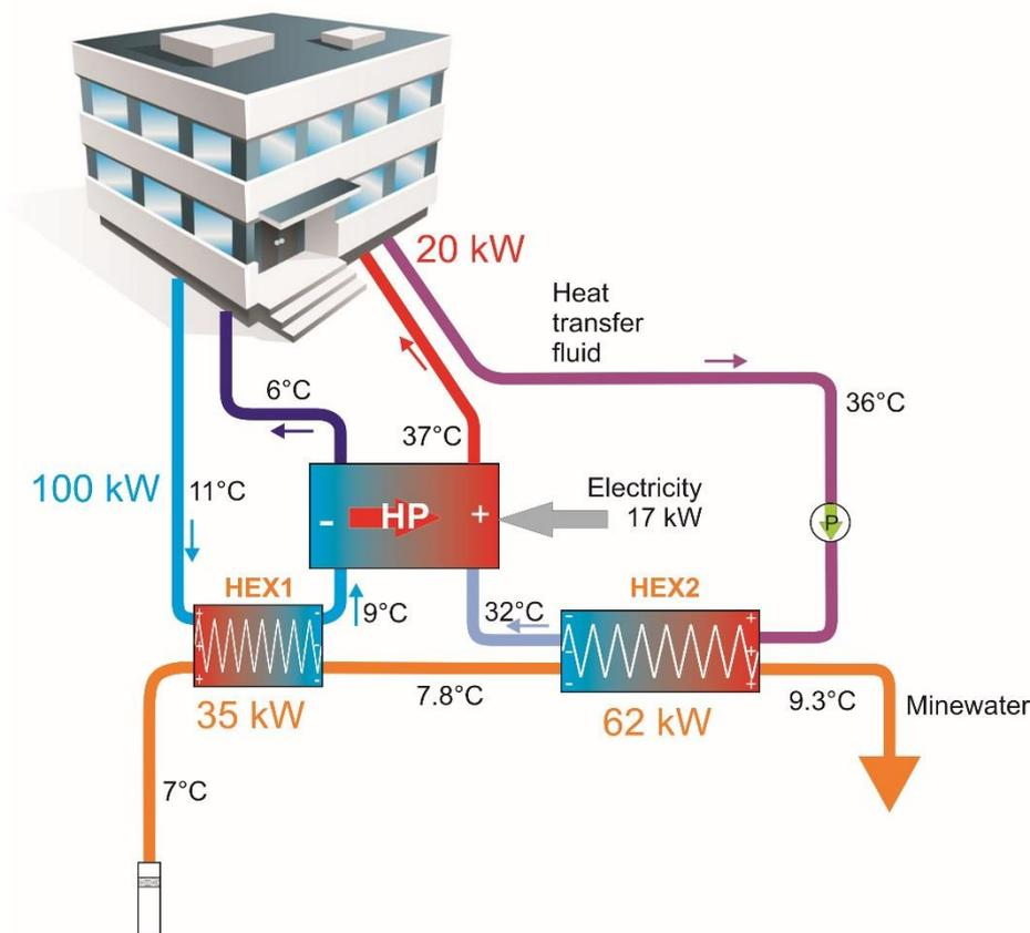
**Figure 3.6.** A schematic example of a mine water heat pump performing cooling, with a subsidiary passive cooling heat exchanger (HEX1) in addition to the “active cooling” heat exchanger (HEX2). Here, the effective COP ( $[\text{heating effect} + \text{cooling effect}] / \text{electricity}$ ) is  $120/17 = 7.1$ .
