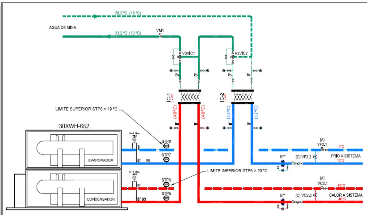
**Figure 6.13. Heat pump GF2 in heating / cooling mode.** In this diagram, cooling dominates heating and the condenser heat exchanger sheds heat to mine water.
