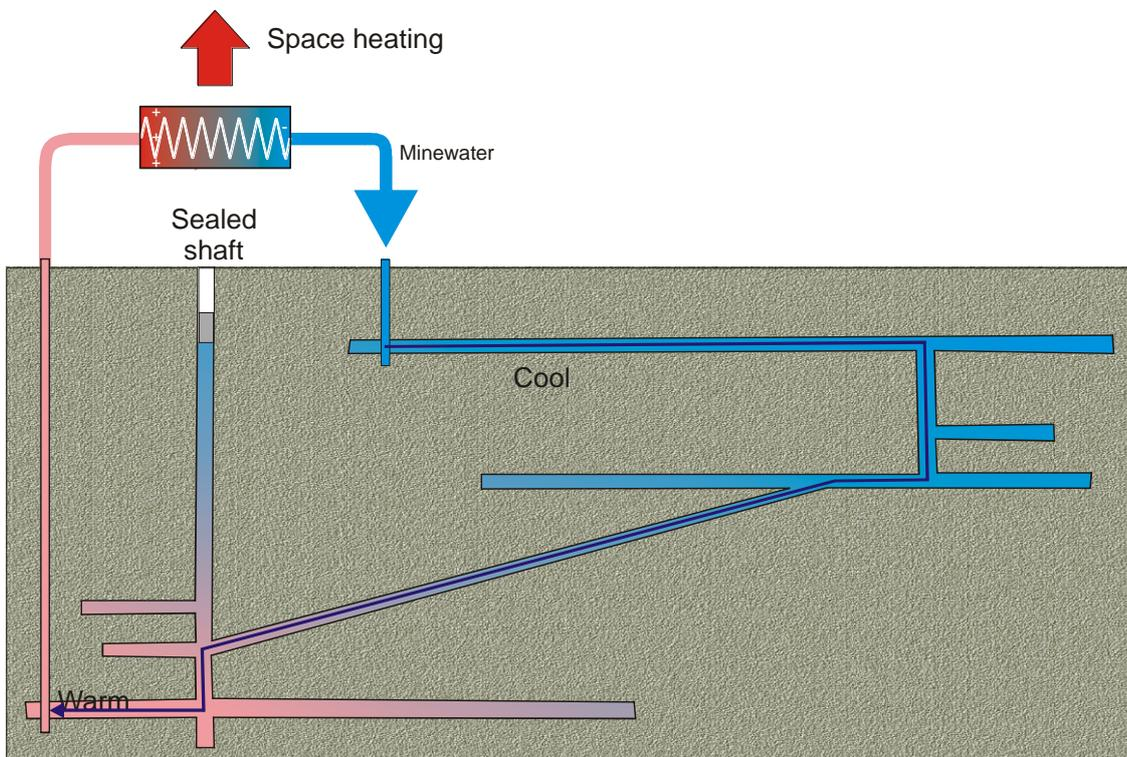
**Figure 5.2. Schematic section of a mine system with deep workings being pumped to provide space heating in winter. The deep blue arrow shows the subsurface flow pathway between the reinjection and abstraction boreholes.**
