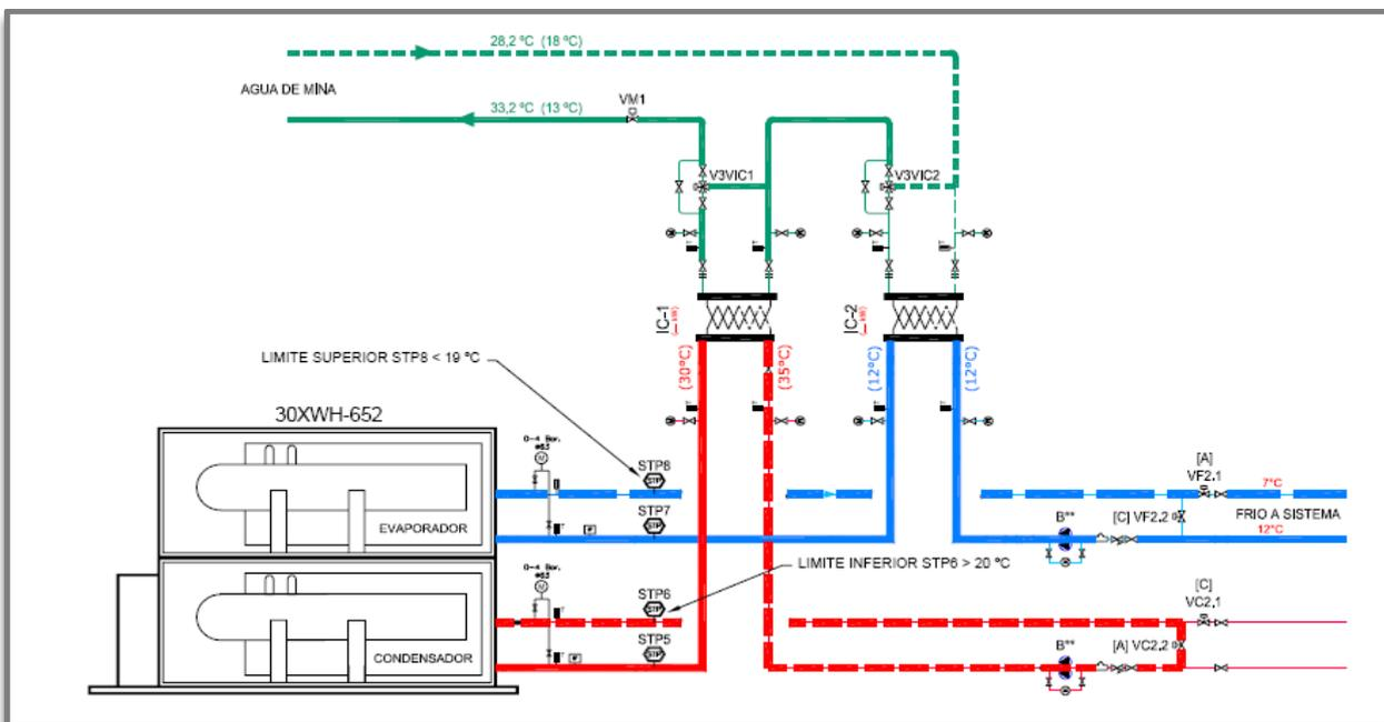
**Figure 6.11. Heat pump GF2 in cooling mode.** Essentially, the condenser of the heat pump is coupled to the secondary heat transfer circuit (and thence to the mine water) via a heat exchanger (IC-1).
